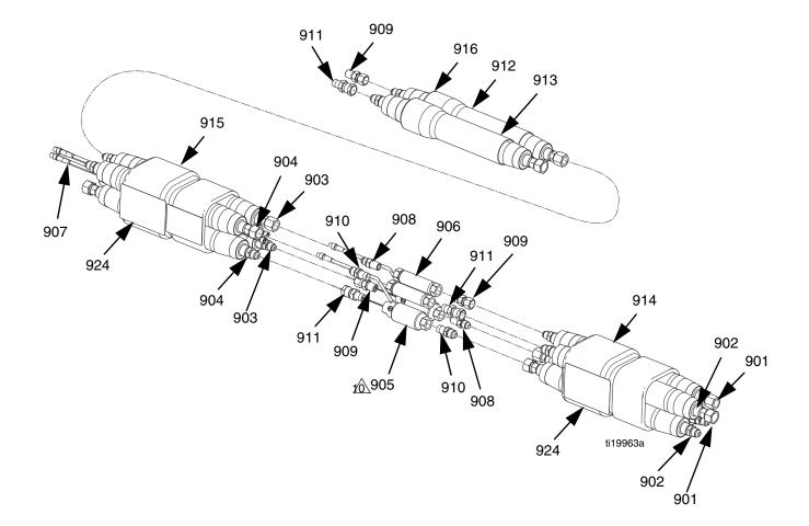
9- Apply pipe sealant to all male threads as needed prior to assembly.
