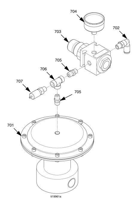
1. Apply pipe sealant to all male threads prior to assembly.
