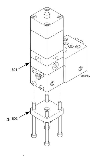
Apply sealant to all male threads prior to assembly. Torque to 3-4 ft-lb (4-5 N•m).
