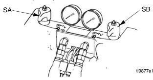
Disconnect the return hoses from the reservoir and secure the hoses to direct flow into a waste container. Cycle the pump at a slow rate until no contamination is seen in either material.
