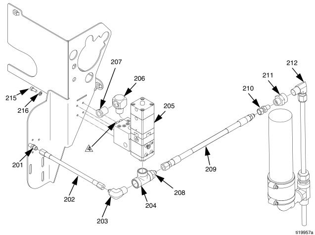
2- Apply pipe sealant to all male threads as needed prior to assembly.
