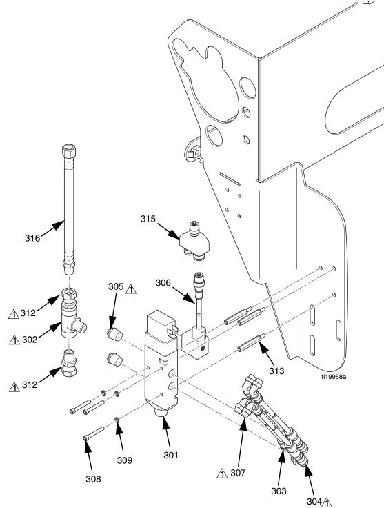
$\triangle$  Apply pipe sealant to all male threads prior to assembly.
